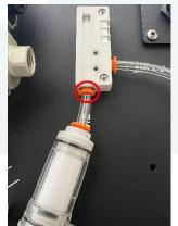
Do this by pushing in the orange ring and pulling the tubing out.
