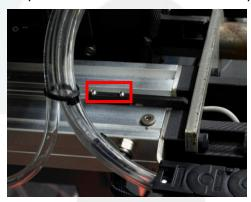
3. Slide the sensor (with retainer) toward or away from the buffer assembly until the sensor's green light is illuminated. Once illuminated, slide it away until the light is no longer illuminated. Move it back toward the buffer assembly just past the point when it illuminates.
